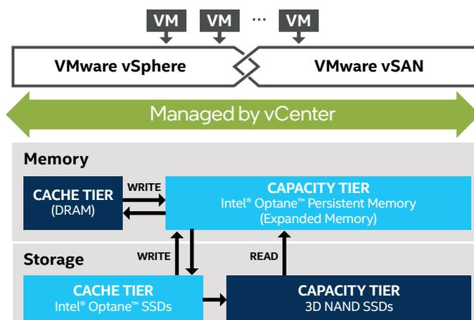
Figure 1. Data moving from memory into the vSAN cache tier and capacity tier.
