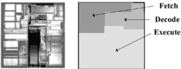
The surface of a Pentium® microprocessor with the fetch, decode, and execute areas indicated.
