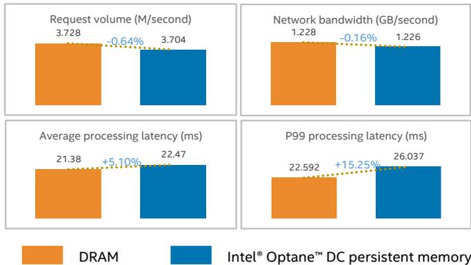
Fig. 4 Pressure test results of the indexing system based on Intel® Optane™ DC persistent memory
