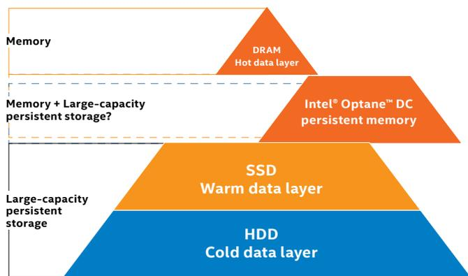
**Fig. 2 Intel® Optane™ DC persistent memory is an ideal choice for both memory performance and large-capacity persistent storage**
