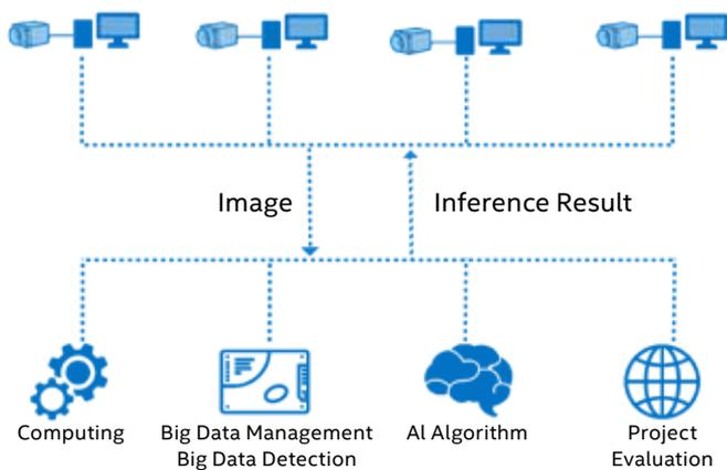
Figure 1. Schematic diagram of Midea's industrial vision detection cloud platform architecture
