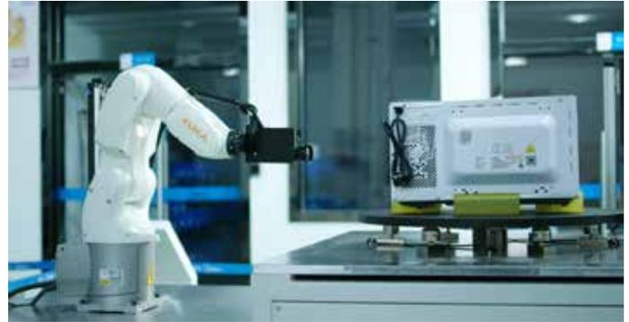
Figure 2. Industrial robot with integrated industrial camera for defect detection
