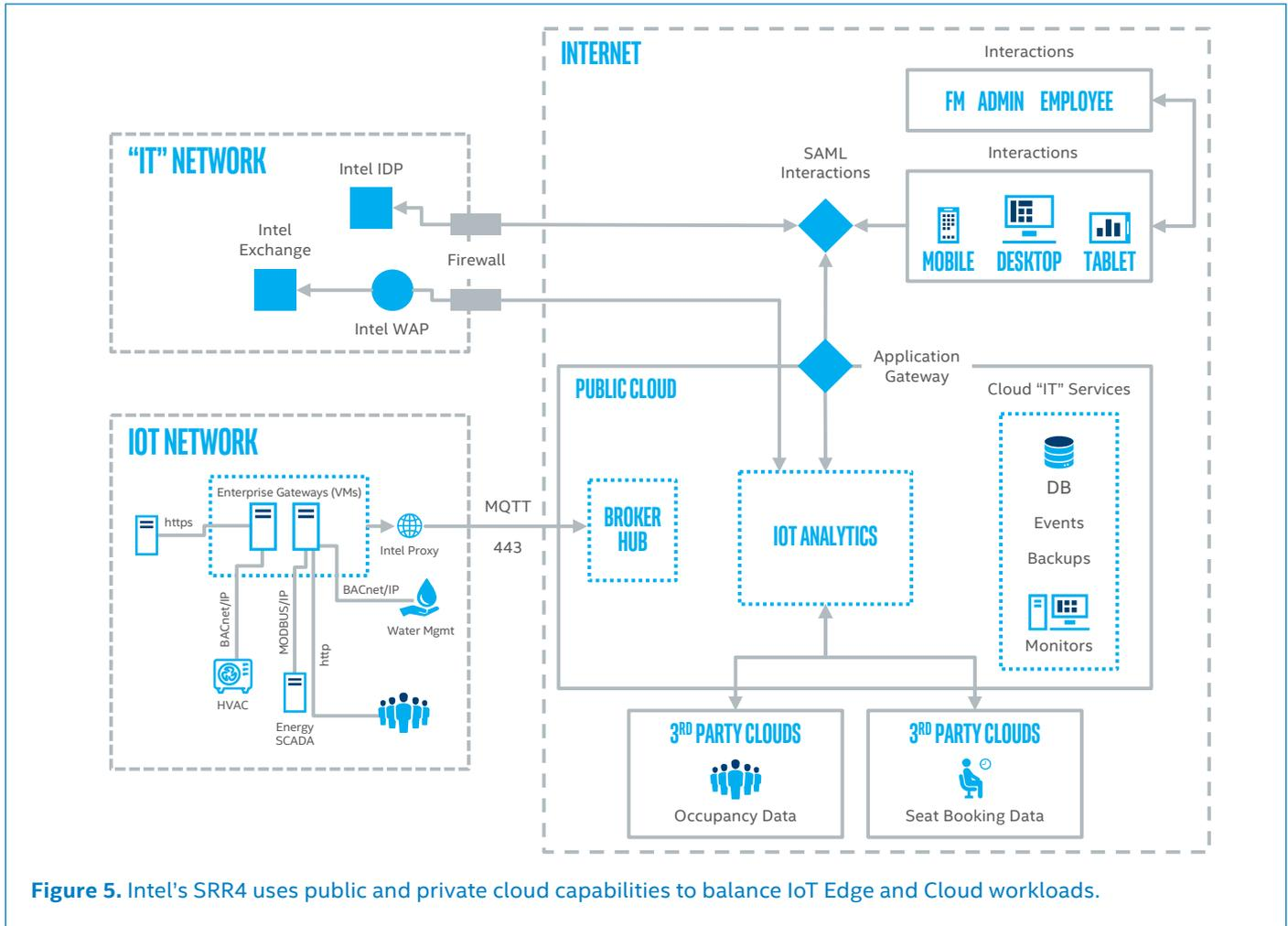
Figure 5. Intel's SRR4 uses public and private cloud capabilities to balance IoT Edge and Cloud workloads.
