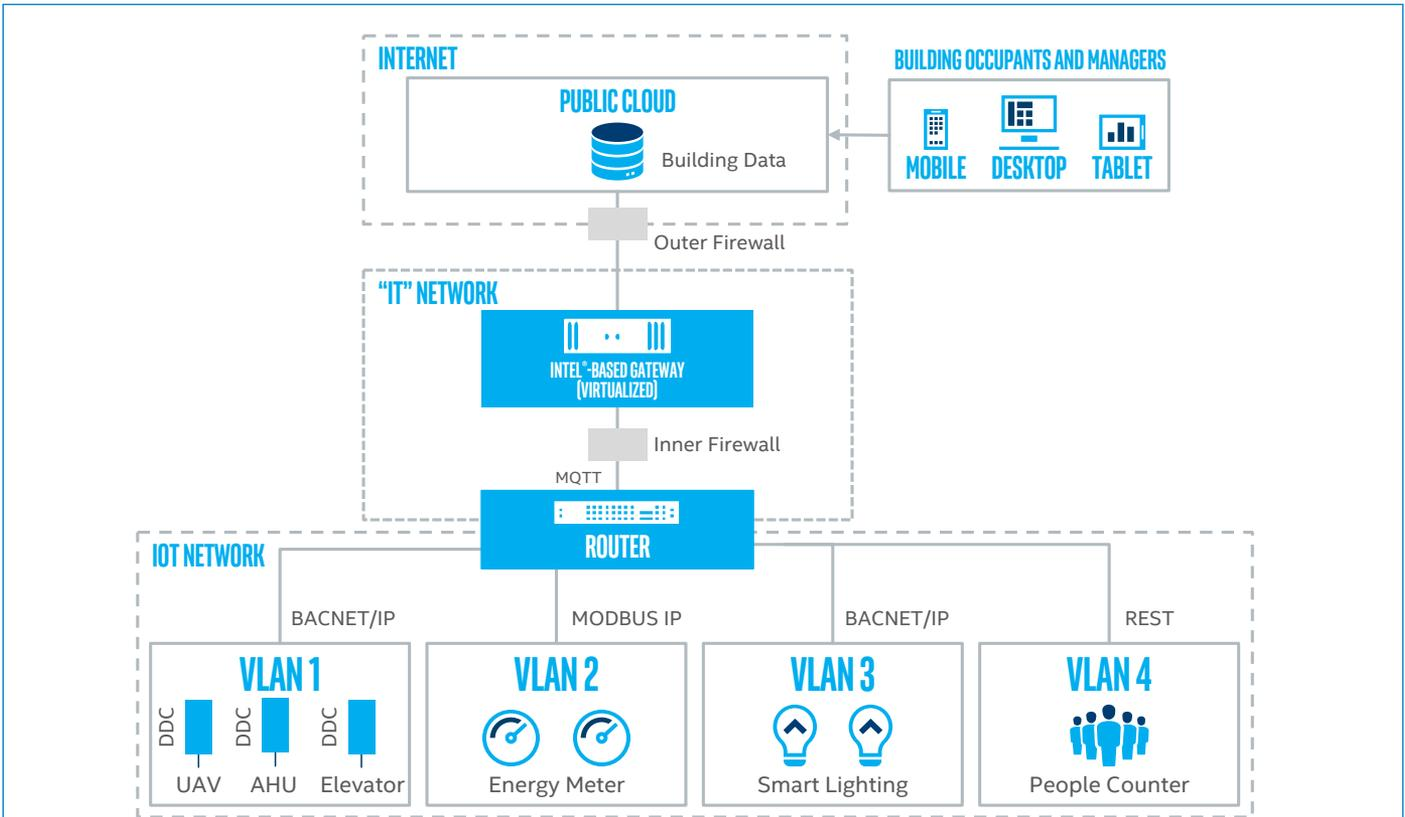
**Figure 4.** The SRR4 network is configured so that Intel IT standardized policies can be implemented across all devices, resulting in improved security overall.
