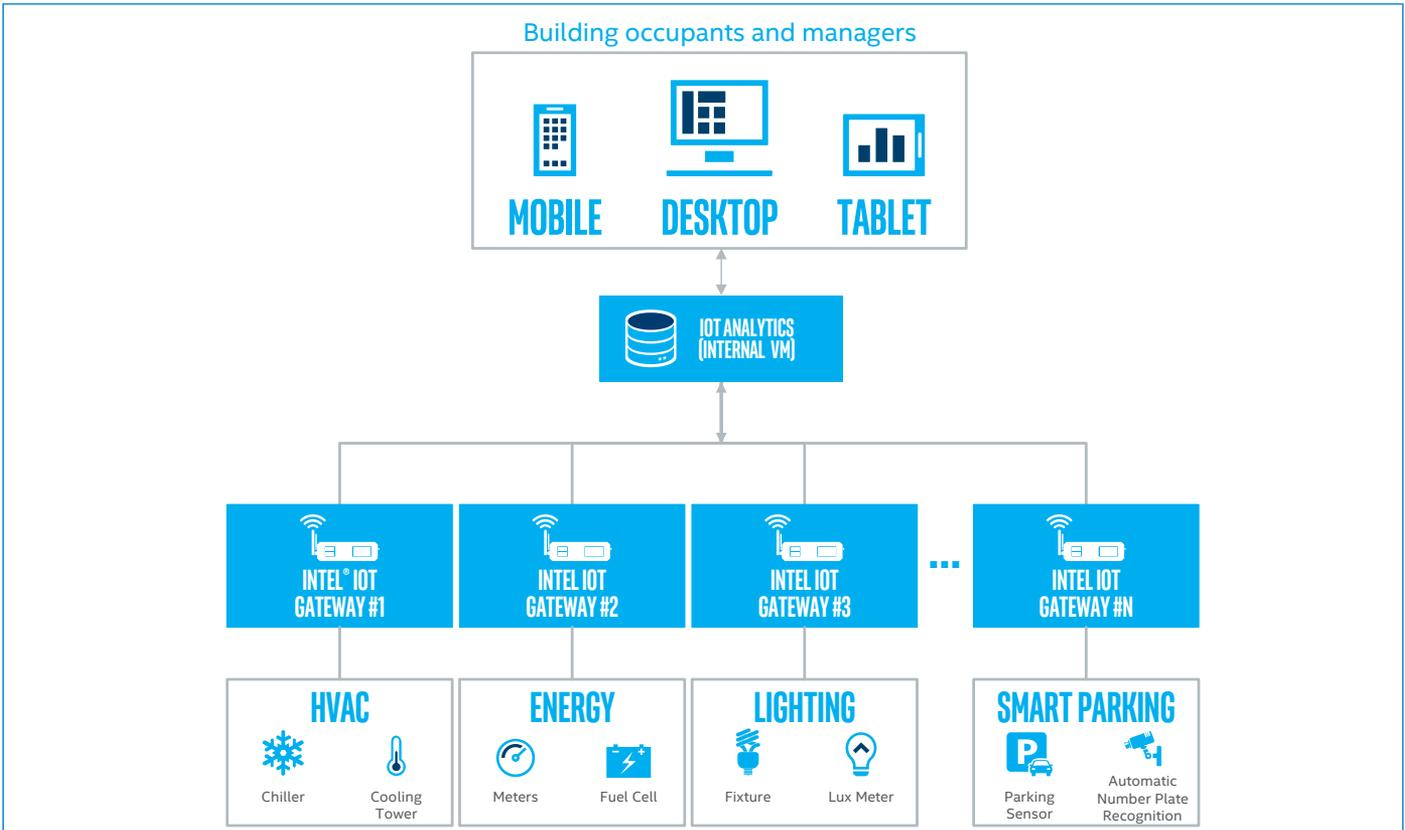
**Figure 3:** The network in Intel's SRR3 smart building in Bangalore, India, places OT devices on entirely separate, isolated networks that are not managed by Intel IT.
