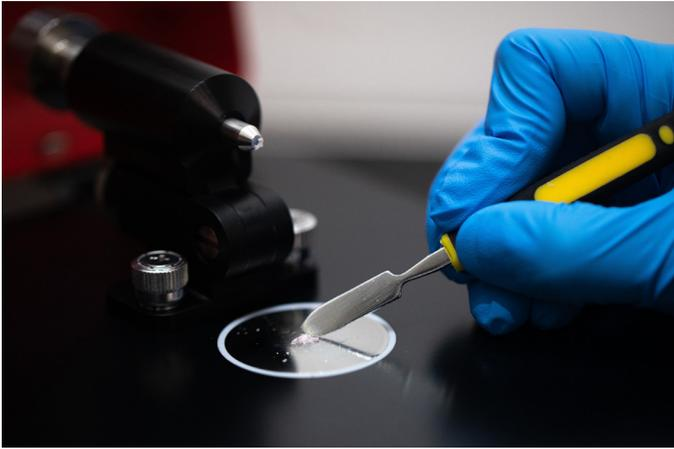
**For infrared absorption spectroscopy measurements, a small quantity of sample is placed on a crystal through which IR light is reflected.** Photo credit: Jay Wallace
