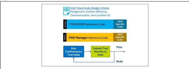
The Intel® RSD Conformance Test Suite (CTS) tool verifies the northbound API schema conformance of the PSME/RMM and PODM through automated techniques. The tool can also test some hardware and software parameters.
