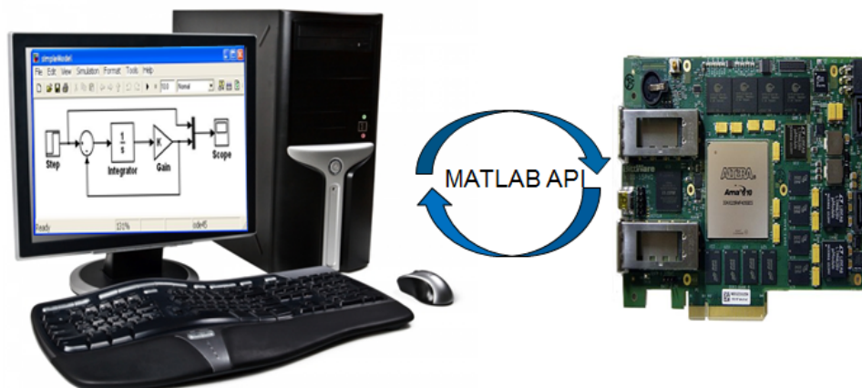
Figure 128. Hardware in the Loop Host-Target Setup
